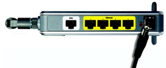
Figure 4-5: Connect the Power
